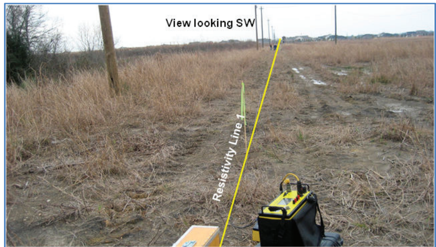
Figure 12. A picture, looking SW, showing the location of resistivity line 1 across Pearland fault.
