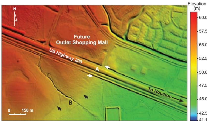
Figure 14. A LiDAR map showing the Hockley Fault location in the vicinity of the study area. The white and black arrows indicate the fault trace at locations A and B, respectively.
