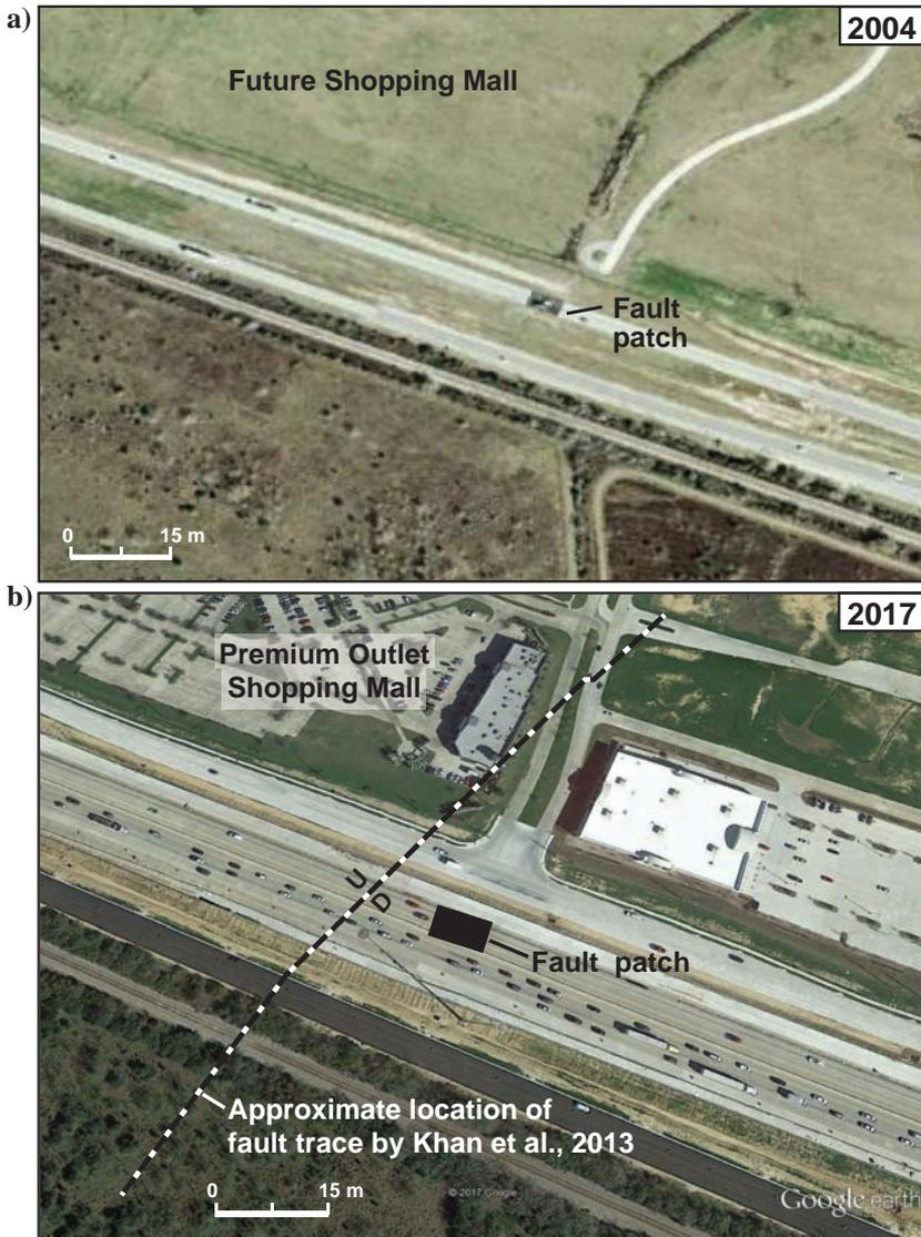
Figure 13. Google images of 2004 and 2017: (a) A patch on the asphalt covers the fault scarp and fault deformation on Highway 290 in the year 2004; (b) the location of the 2004 patch is plotted on the 2017 Goggle image. The fault trace obtained by Khan et al. (2013) is also shown on the site map.
